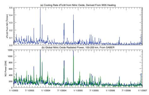
**Figure 4.** Results from the revised thermosphere temperature calculation described here for the years 2003 through 2006. (a) The blue line shows the cooling rate of the thermosphere due to the effect of NO. These are the same as in Figure 3c, except the longer time period is shown and the 24 h smoothing has already been applied. (b) The green and blue lines are the same as in Figure 3c, using the fit in equation (11) for this longer time interval.
