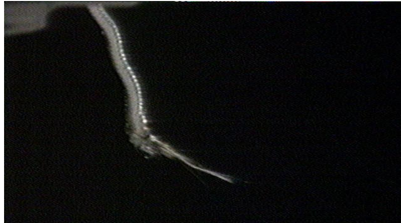
Figure C.8 — The end of the remaining TSS-1R tether (Ferguson and Hillard, 2003, p. 27)
