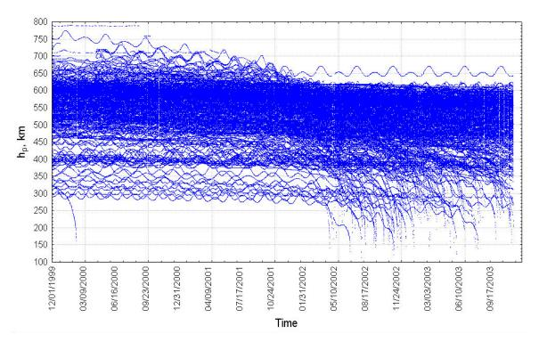
Figure 1 — Time-altitude distribution of ballistic coefficient estimates (for all SOs) 2000 – 2003
