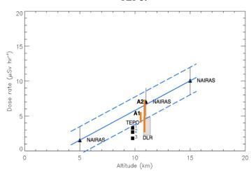
Figure 8. Dose equivalent rate comparison for NAIRAS (triangles), TEPC (squares), ARMAS FM (A1 and A2 orange bars), and DLR DUS-MRU TEPC (gray rectangle).
