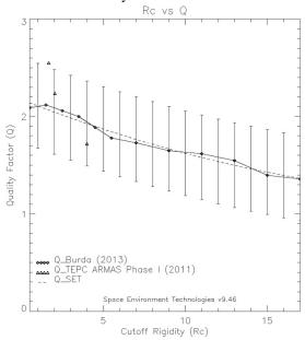
Figure 4. Qset as the dashed line fit to the Burda measurements of Quality factor (Q) (diamonds with error bars) and validated with Gersey TEPC data (triangles).
