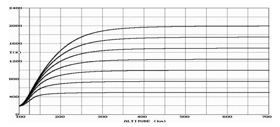
Figure 4. Temperature Profiles ( $T_{\infty} = 500, 750, 1000, 1250, 1500, 1750, 2000$ °K with  $\Delta T_{x} = 0$ )
