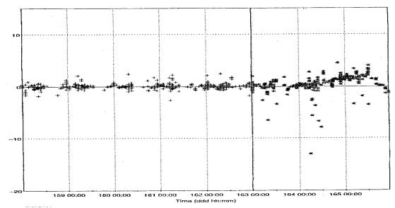
Figure 3. In-Track Residuals for a LEO Satellite (5-Day Segmented Fit / 3-Day Prediction)
