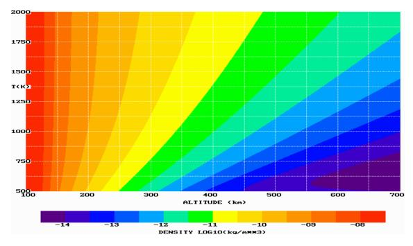
Figure 6. Density versus Altitude and Exospheric Temperature  $T_{\infty}$  (with  $\Delta T_{\rm x} = 0$ )
