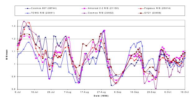
Figure 1. Scaled Ballistic Coefficient Histories ( $B_{\text{scale}} = B_{\text{model}} / B_{\text{true}}$ )
