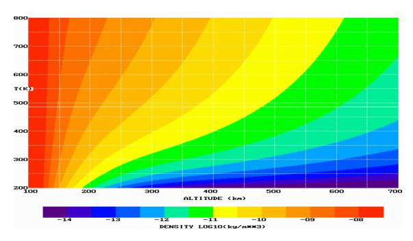
Figure 7. Density versus Altitude and Inflection Temperature  $T'_x$  (with  $T_\infty = 2000$ °K)
