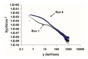
Fig. 4. Frequency distribution of SEPCM lineal energy spectra normalized per incident neutron per cm<sup>2</sup>.
