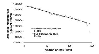
Fig. 1. Differential neutron flux at LANSCE ICE House facility, and neutron flux found in the atmosphere at an altitude of  $12\,000$  m multiplied by  $3\times10^5$ .
