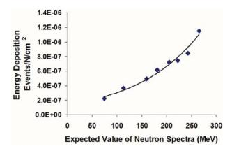
Fig. 6. Number of energy deposition events per neutron per  $\rm cm^2$  with lineal energy greater than 1000 keV/micrometer as a function of expected value of the incident neutrons energy spectra. The solid black line is the result of a least squares regression of the data points.
