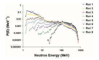
Fig. 3. Differential probability distribution of neutron energy spectra used in experimental Run 1 through Run 8.
