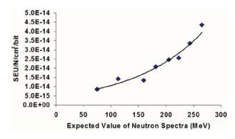
Fig. 5. SEU cross sections as a function of expected value of the incident neutrons energy spectra. The solid black line is the result of a least squares regression of the data points.
