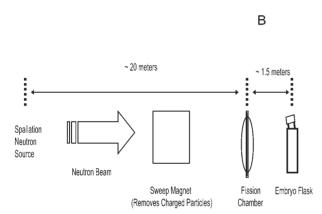
FIG. 1. Panel A: Differential energy spectrum of the LANSCE/WNR neutron beam line used in this study, and neutron flux found at an altitude of 12,000 m in the atmosphere. Panel B: Medaka irradiation using the 30L LANSCE/WNR neutron beam line. Relative positions of the neutron source, sweep magnet, fission chamber and embryo flask are shown (figure is not to scale). In some experiments, a TEPC was placed in line behind the embryo flask for dosimetry purposes.
