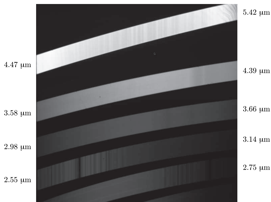
Figure 5.5: A flat-field taken with SpeX using the LXD2.3 mode. Indicated is the approximate start and end wavelength of the different orders. After Rayner et al. [2003].
