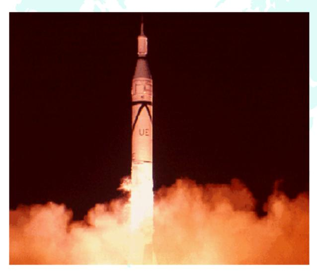
Explorer 1 carried one instrument, a Geiger counter, designed to observe cosmic rays. The experiment worked well at low altitudes but counted no particles at high altitudes.
